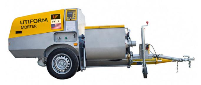
Diesel screw pump, with a powerful 19 kw STAGE V engine. Complies with current emissions regulations, established for the European Union.
